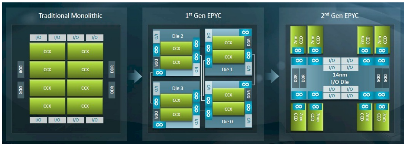
Figure 1. Monolithic, Naples and Rome CPU layouts, from
