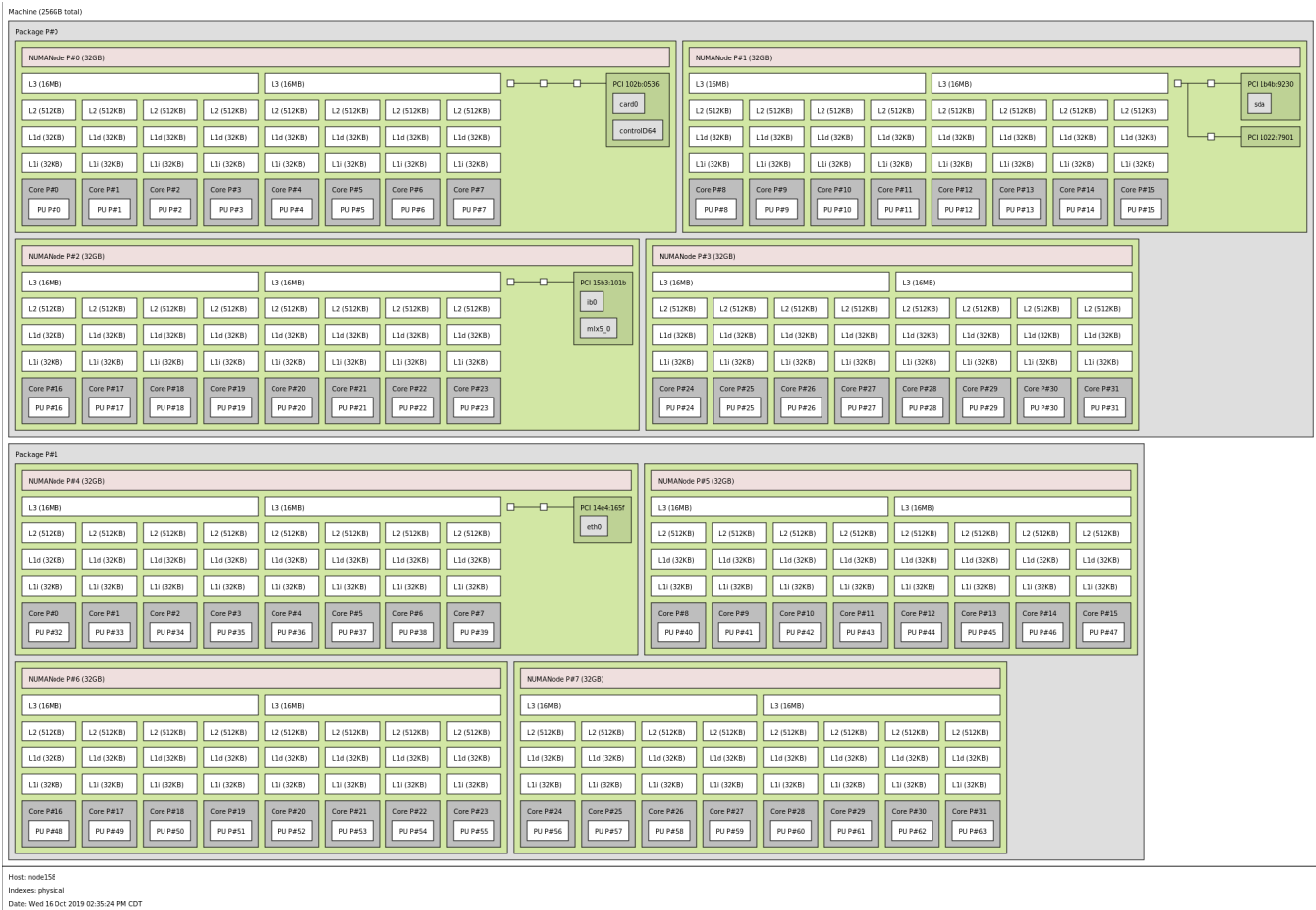
Figure 3b. NUMA layout of a 2x32 core (2x EPYC 7452) Rome server in the dual NUMA level mode. Package is the CPU, NUMANode are the CCDs. Each L3 cache is shared by 4 cores marking the CCX.
